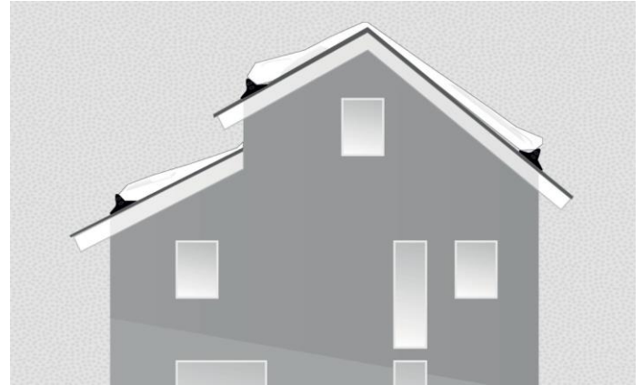
Snow guards are installed on each slope of multi-level roofs
